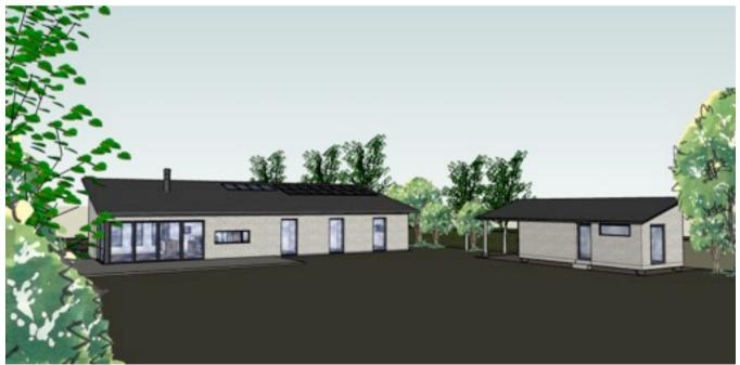
The decision was made to clad the exterior in Scottish larch, complete with a Tata seam steel roof, while carefully positioned glazing breaks up the timber to capture the views over rolling fields to the south and of Ben Wyvis to the north. The large glazed sections allow heat and light into the building which helps create a warm and bright living space.
